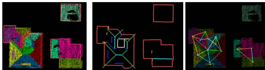
Figure 5-14 Roof segments (left), intersection lines and step edges (middle) and roof topology graph (right).
