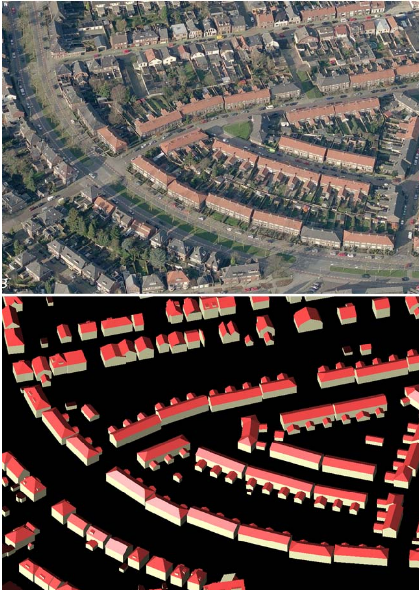
Figure 7-11 Comparing oblique image of Indische buurt area with reconstructed models. Image taken from Bing.com.
