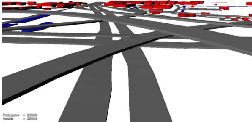
Figure 3-13 Four levels of highways have been reconstructed automatically.
