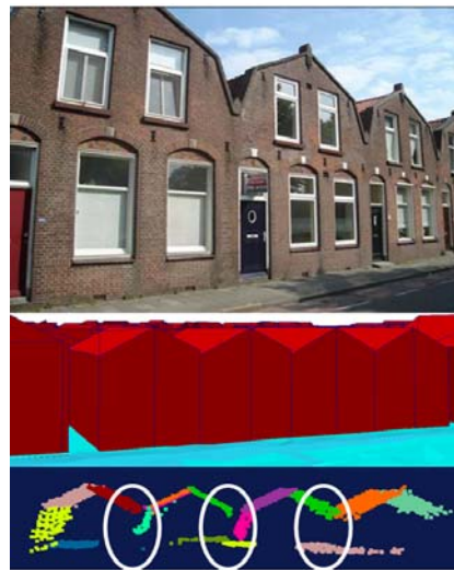
Figure 5-6 Gambrel roof types (top) are often modelled as gable roofs (middle), caused by missing laser segments at the lower roof faces of the gambrel roof (bottom) because of occlusion by the higher roofs.
